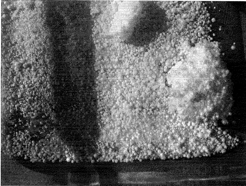
Figure 1. Visible failure of silica gel to properly foam to form spheres due to usage of a non-rotary furnace.
